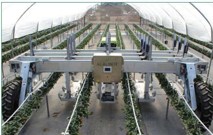
The Agrobot has mechanical arms to pick strawberries that are trained to grow for machine picking.
