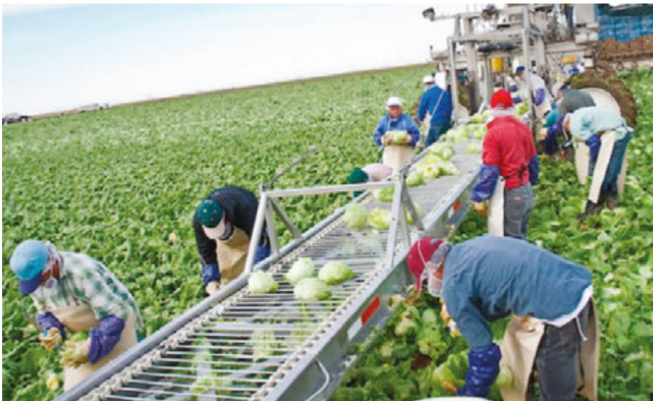
Photo 4. Conveyor belts for harvested produce and packing for market in the fields means higher productivity for workers and less handling of produce.
